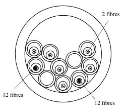
Figure 7 Cross-sectional view of tubes and cables for network-structure of Figure 6.
